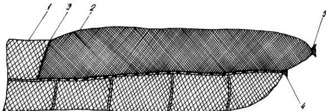
Fig. 3.8.2. Codend bag scheme: 1 - main bag 2 - apron; 3 - connector, 4 - the main bag 5 - the trailer outer bag connection
