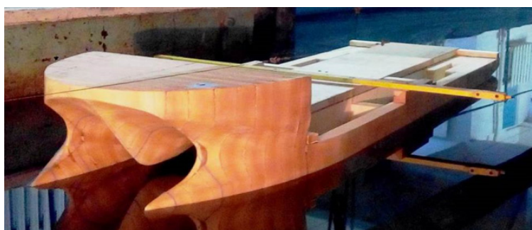
Fig. 3. Model before harnessing to the pool towing system
