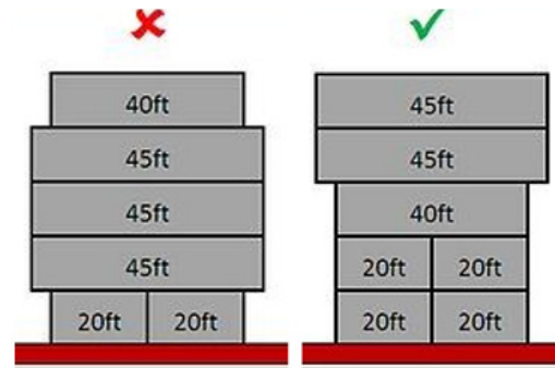
Fig. 11. Wrong and correct stowage of 45ft containers ( https://www.container-logic.com/single-post/2016/02/17/Container-Types-Part-2 )
