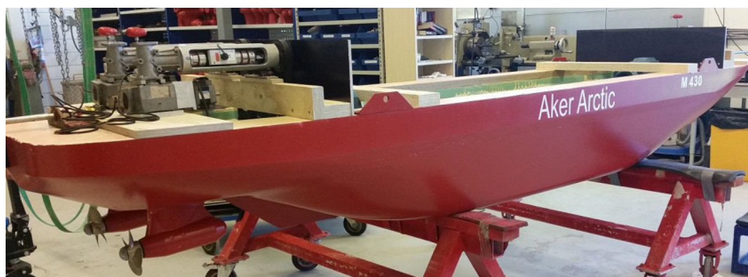
Fig. 2. IBSV01 hull model developed in the Aker Arctic ice tank
