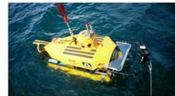
The 3-person submersible PC-8B , equipped with a scanning sonar, lights, an underwater video camera, and manipulator, is capable of diving to depths of 250 meters.
